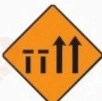
Two nearside lanes (of four) closed
