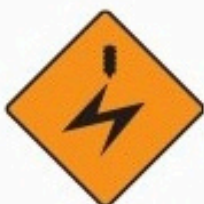
Overhead electric cables
