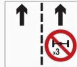
In a tunnel goods vehicles cannot use right-hand lane (by reference to number of axes)
