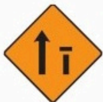
Offside lane (of two) closed
