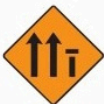
Offside lane (of three) closed
