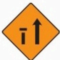
Nearside lane (of two) closed
