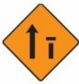
Offside lane (of two) closed
