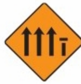
Offside lane (of four) closed
