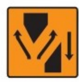
Lanes diverge at crossover
