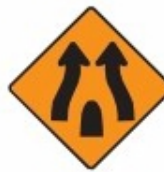
End of obstruction between lanes
