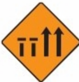
Two nearside lanes (of four) closed
