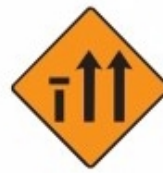
Nearside lane (of three) closed
