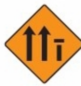
Offside lane (of three) closed
